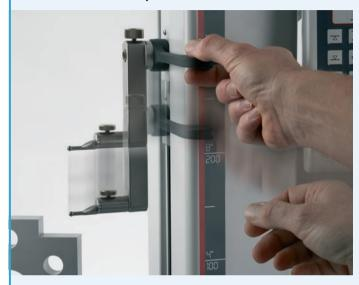
1. Move the measuring carriage by hand in the direction of the object to be measured.
