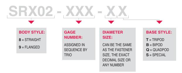
Trulok<sup>®</sup> gages are built to your exact specifications. Please supply us with the following data needed for the calibration set block that will accompany the gage:
