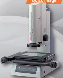
Camera based profile profile projector featuring automatic edge detection software.
